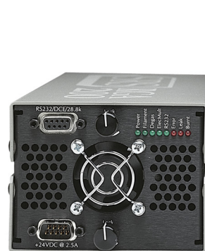
CIS rear panel (without AC power module)
