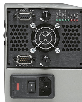
CIS rear panel (with AC power module)
