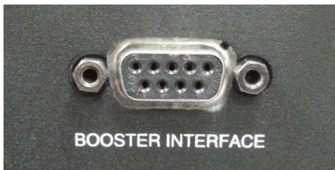
Figure 28: Rear panel connector for booster interface.
