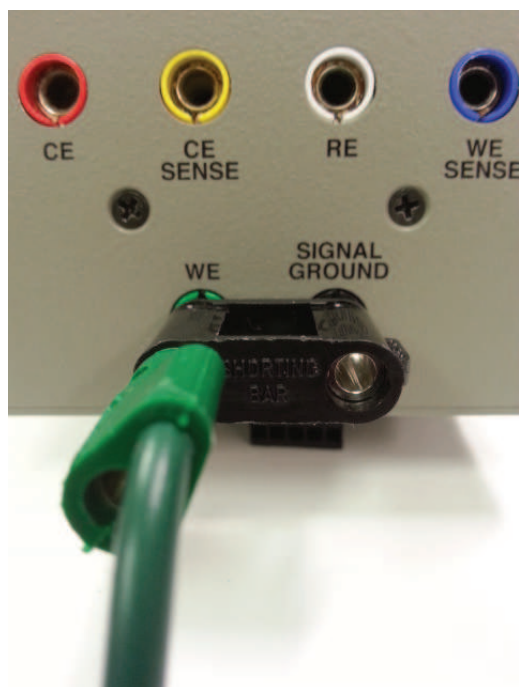
Figure 15: Grounding WE at the EC19.
