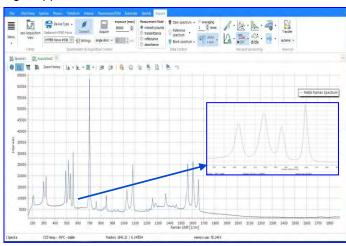
HYPER-Nova Spectrometer configured for 785nm Raman measuring our Maltol Standard Sample. Zooming in on one of the characteristic quadruplets shows the amazing low noise characteristics of this new spectrometer system
