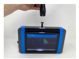
White LED Color: white light comes in a variety of flavors - warm, cool, incandescent, LEDs. The StellarRAD automatically calculates CCT and CRI. Easily distinguish and compare white LEDs.
