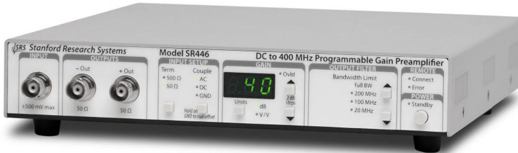
The SR446 is a single-channel, 400MHz bandwidth voltage preamplifier with 21 programmable gains from 1 to 100 (+0 dB to +40 dB with 2 dB steps). It also includes four programmable low-pass filters, with settings of full bandwidth, 200 MHz, 100 MHz and 20 MHz. There are two output channels which offer complementary outputs (inverting and non-inverting) that can be used separately, or together as a differential output.
