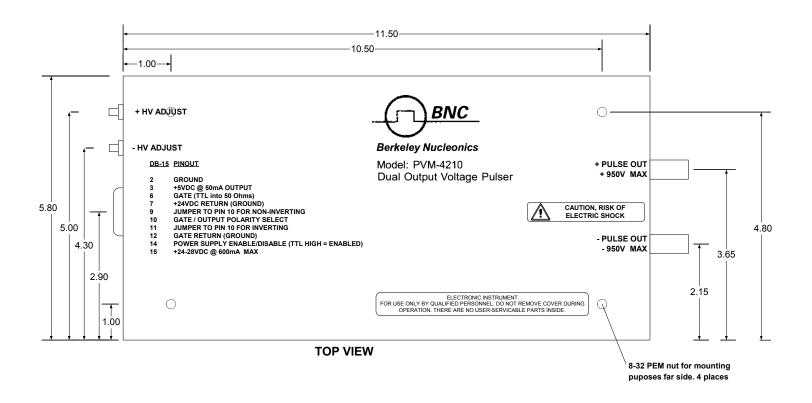
PVM-4210 Mechanical Dimensions And Mounting Hole/Connector Locations
