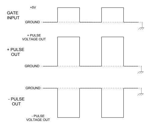
Output Pulse Configuration With Non-Inverted Gate Selected
