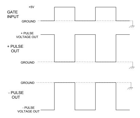
Output Pulse Configuration With Inverted Gate Selected
