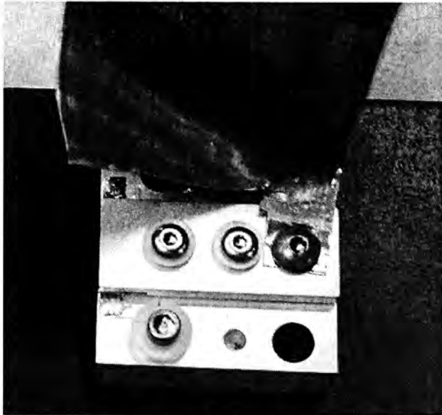
Figure 5 - Stripline Connection To Laser Diode
